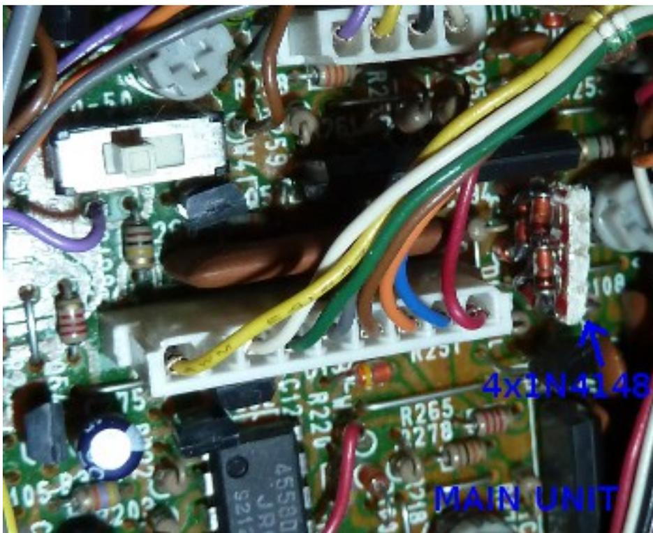
This modification makes the power increase about 2 times, but the drawback is that the PA might be more easily destroyed.
