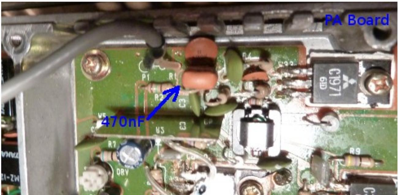
*PA board coupling capacitor modification*
